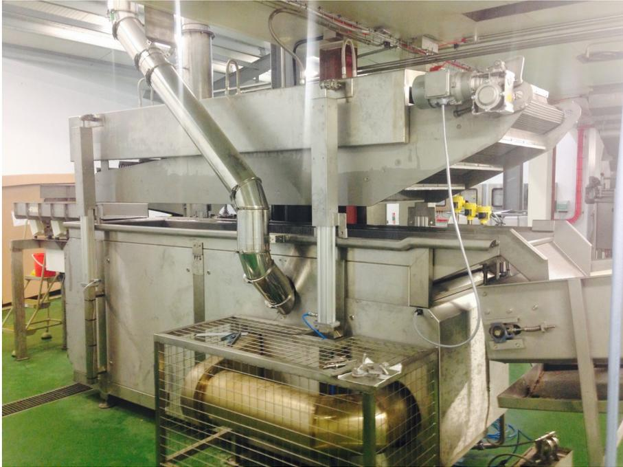
Fabcon manufactures a range of fryers for snack pellets made from a wide variety of grains such as wheat, rice, tapioca, cassava etc, or potatoes, other vegetables and pulses in 2D or 3D shapes.
